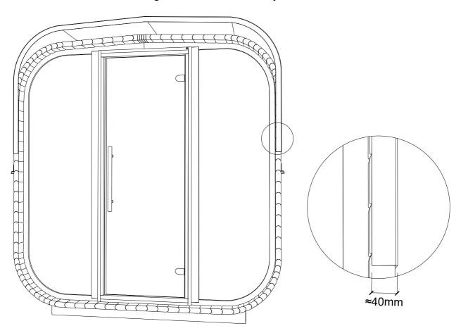
STEP 29: Staple underlay at the front and back edges. Cut excess underlay if necessary.
