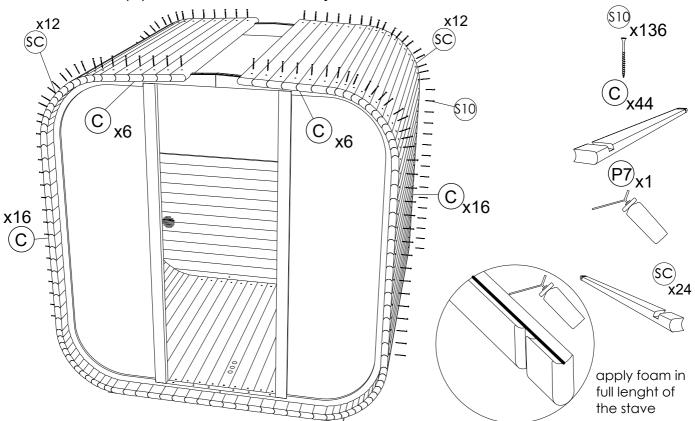
**STEP 15**:Finish roof with the 2 (C) staves and final staves (H). If needed, use thinner staves (H1) to fil the gap between (H) staves and apply foam between staves. Make sure that centre of the roof is tightly filled, then fix with screws (S10) 4x60.
