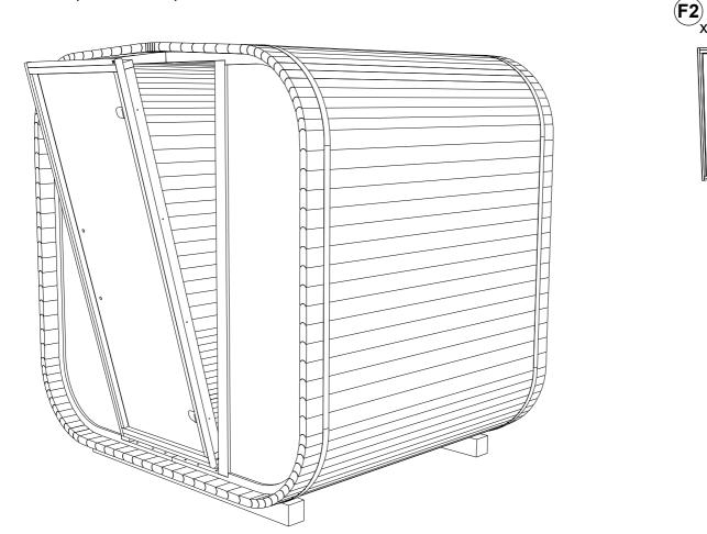
**STEP 19:** Put plastic spacers in the gap between the door box and the front panel where the screws go. Combine spacers for best width. Spacer must fit tightly.
