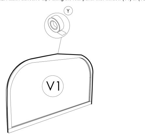
**STEP 13**: Install the panoramic panel (V1) with caution. Use foam between panels for better insulation. Place it on top of the lower back panel (V). Check level and that side edges are aligned with bottom panel. One keeps holding the panel, and the other is fixing the side stave on a curve using screws 4x60(S10). Secure the panel (V1)with screws at the both corners
