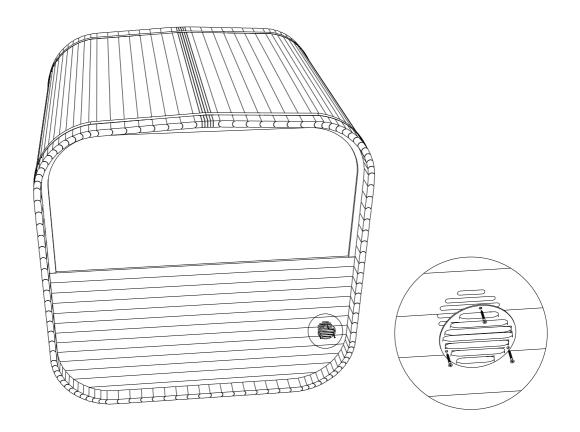
**STEP 18:** Install the doors (F2). Put the doors on threshold and lay in frame about in the middle. Fix doors with clamps or another person should hold the door.
