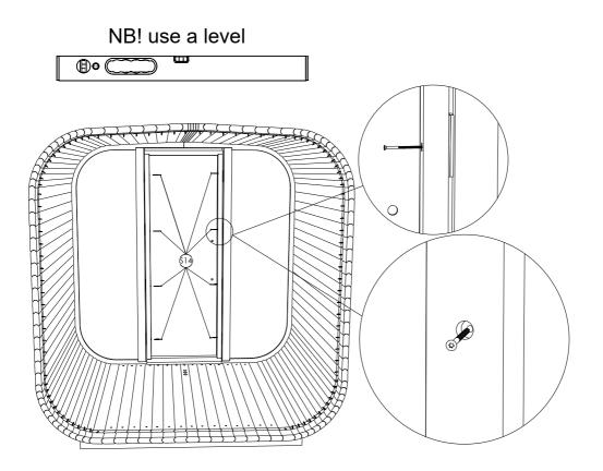
**STEP 21:** Use foam around door box. Don't clean up the foam until it's dried out. The excess amount will come off easily if you don't touch it while it's wet. Fix door moldings to both sides and on top of the door with (S5) screws 4x50ss.
