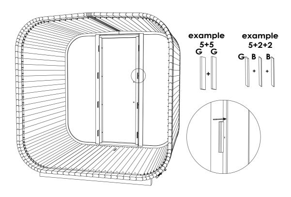
**STEP 20:** Fix one side of the door box with screws 5x80 (S14) slightly to the outside through spacers. Then put spacers in other side. Combine spacers for necessary width. Spacers must fit tightly, they can't slip down before door is fixed with screws. Use screws 5x80 (S14) to fix doors. Check door box, both sides should be straight, they must not be bent inwards or outwards.
