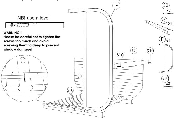
**STEP 8**: Place the second front panel (F). Slid it together that the top and bottom conects. Fix it at the panel treshold with screws 4.0x70(S2). Make sure it's level. Use metal bracket on top of the front panels to fix them together.
