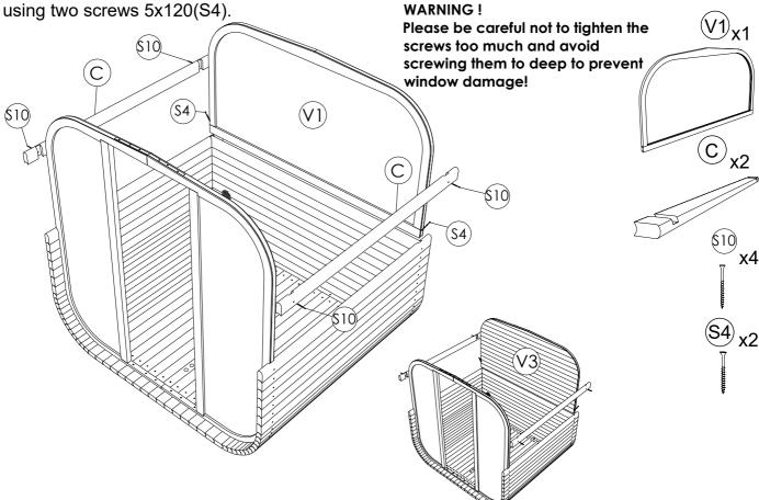
**STEP 14**:Fix 16 staves (C) on both sides using 4x60 (S10) screws. Use a rubber hammer for tighter placement. On the arches use 12 (SC) staves on both corners using 4x60 (S10) screws. Fix last 6 staves (C) Use foam between every stave.
