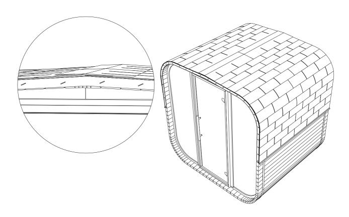
**STEP 36:** For top of the roof use starting shingles. Cut some shingles in squares, there are marked lines. Take off protective film. Nail each shingle with two nails. Next shingle goes about 160mm over previous. After it's done, use heat source for better adhesion.
