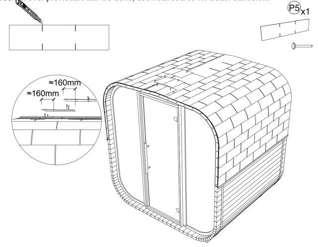
**STEP 37:** Install front and back decorative roof finishing boards using (S7) screws 4.2x55 brown. Start by fixing two top boards, then rest of it goes next to each other.
