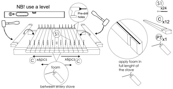
**STEP3:** Drill fourteen 10mm holes in front and back wall groove to the out-side in board connections as shown in the picture.
