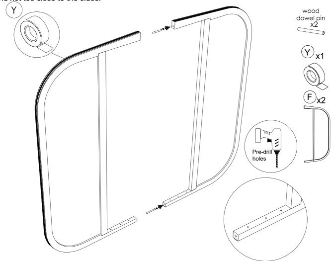
**STEP 7**: Draw a line on the center stave where the middle is. Take one of the panels (F) and put it directly next to the middle line. Take one stave to connect both panels, front and back, using screws 4x60(S10). Fix it at the panel treshold with screws 4.0x70(S2). Make sure it's level.
