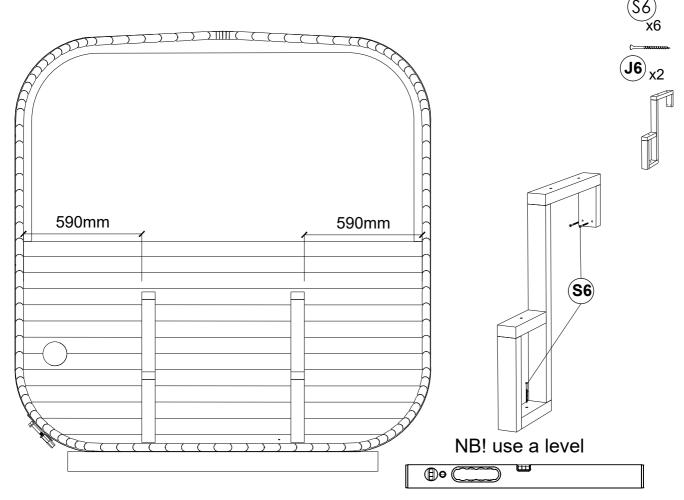
STEP 23: Place long sauna bench upwards on the bench legs. Then install bench support boards (J3) on the side walls using S6 screws 5x70SS, at the same level as the bench legs. leave gap from back wall about 20mm.
