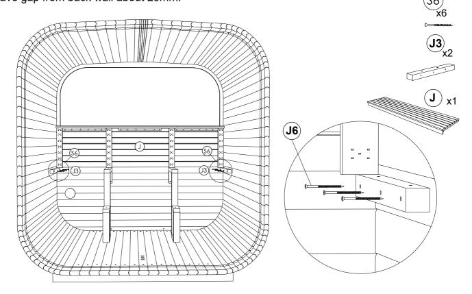
**STEP 24**: Install sauna bench (J) on top of the legs (J6) using (S6) screws 5x70SS. Bench cross boards have to match the tops of the bench legs. Fix Bench step (J4) using (S6) screws 5x70SS.
