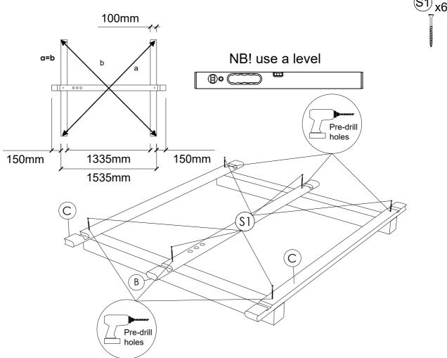
**STEP 2:** Fix 10 staves (C) to each side from the center stave. Check level while installing staves and use rubber hammer for tighter placement. Pre-drill holes for screws. Use foam between boards for better insulation.
