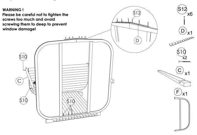
**STEP 9**: Fix one stave (C) on both sides with screws 4x60 (S10). Use rubber hammer for tighter placement. Use foam between every stave. When both corners are done, take of connecting staves. Keep fixing staves till reach top of the rear panel (V). Fix ventilation grill from outside on ventilation cuts and air diffuser from inside.
