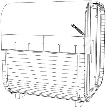
**STEP 32:** Remove the protective film from the bottom of the sheet. The second row starts with the whole shingle, fix it with shingle nails.
