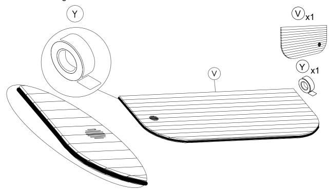
**STEP 5**:Place rear bottom panel (V) in the board grove. Check that the panel is level. Secure panel with screws 4.0x60 (S10) at the both corners through the stave.
