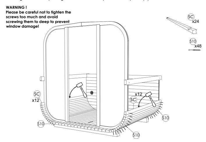
**STEP 11**: Fix one stave (C) on both sides with screws 4x60 (S10). Use rubber hammer for tighter placement. Use foam between every stave. When both corners are done, take of connecting staves. Keep fixing staves till reach top of the rear panel (V).
