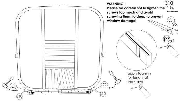
**STEP 10**: Fix 12 stave (SC) on both sides with screws 4x60 (S10). Use rubber hammer for tighter placement. Use foam between every stave. When both corners are done, take of connecting staves. Keep fixing staves till reach top of the rear panel (V).
