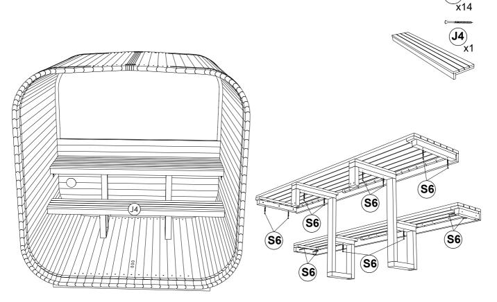
**STEP 25**: The left leg leg needs to be installed next the front panel (F), right leg is 750mm from bottom rear panel.
