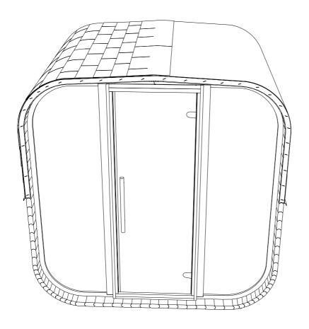
**STEP 35:** Repeat same steps for other side, till last layer goes over middle of the roof. Use heat source for better adhesion. Lift every rectangle, heat a bit and press it to the roof.
